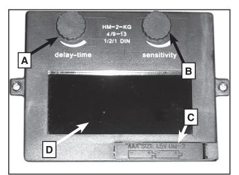
Figure 2. View of the inside control panel.
